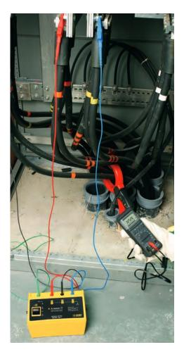
Generates a momentary grounded artificial neutral to allow the measurement of fault currents on ungrounded three-phase systems
