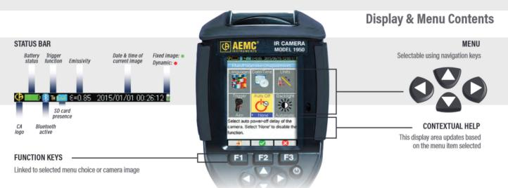
A comprehensive set of easy access menus are available on screen. You can use the function and navigation keys to easily configure the camera for your specific needs. Trigger functions can be programmed, color palettes can be selected, cursor tools can be configured as well as environmental conditions including ambient temperature and humidity, distance and emissivity.
