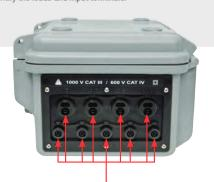
The voltage and current inputs, as well as the power cord connection are constructed with screw on, watertight connectors rated to IP67.
