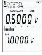
**AREL MODE** Displays relative values with respect to referenced measured value
