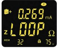
Detects and displays possible false readings associated with metal loops
