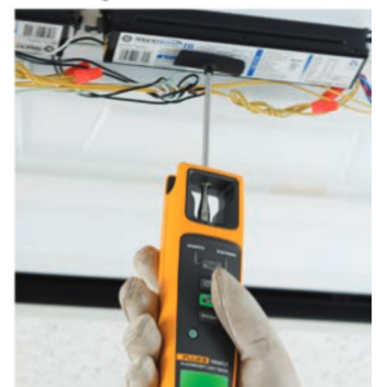
Easily determine if ballast is working.
