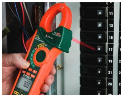
Built-in IR Thermometer for quick and safe non-contact temperature measurements.
