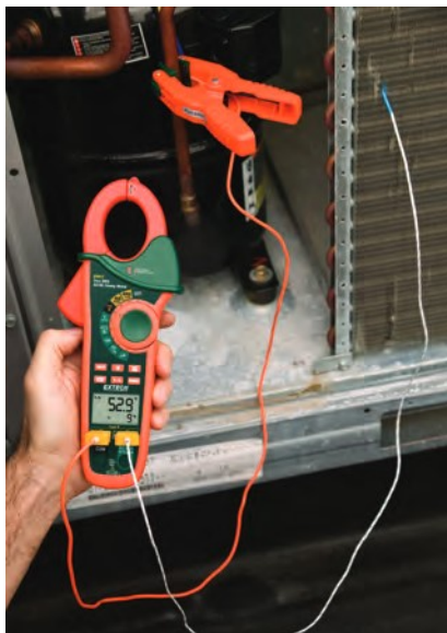
Dual Type K Inputs for taking differential temperature readings needed for superheat measurements.
