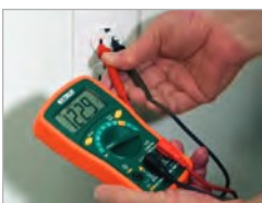
Displays AC Voltage of an outlet receptacle
